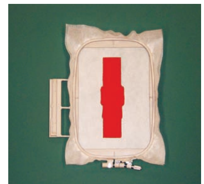
Color 3: Tacks down the edges of the appliqué with an overlapping zigzag stitch.
